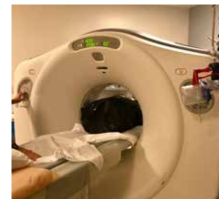
An occupied log being scanned by the CT machine.
